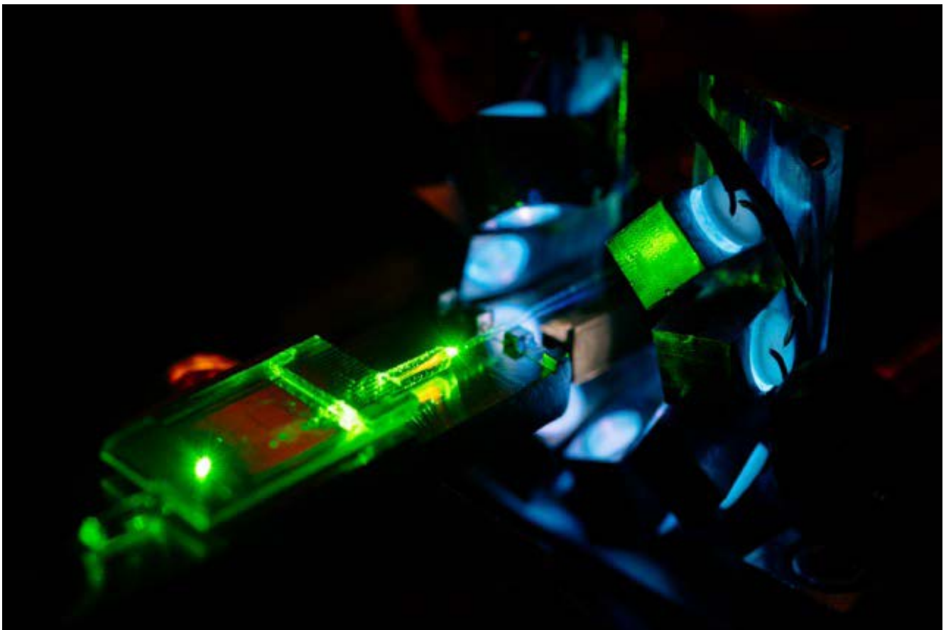
Pigtailing. Optical fibres are attached to our samples to provide hands-off operation. (UPB, Besim Mazhiqui)
